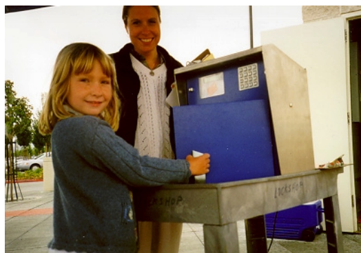
A girl checks a vehicle key into the CarLink key manager using a smart card.
